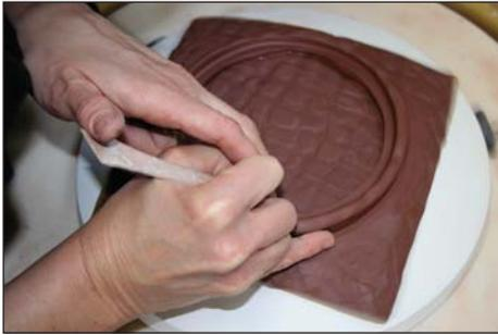
19. With wheel turning, trim coil to make level foot using a Trimming tool.
